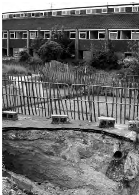
Figure 3.17. One of the collapse sinkholes formed by liquefaction failure of the chalk over old mines in Bury St. Edmunds, U.K., seven years after their failure destroyed the road. TW.
