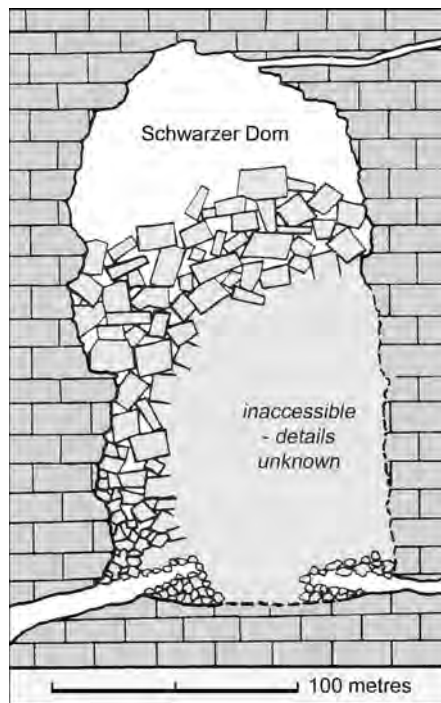
Figure 3.27. Cross section through the Schwarzer Dom in Hölloch, Switzerland, where progressive collapse of a cave roof has produced a short breccia pipe. After Bögli (1980).
